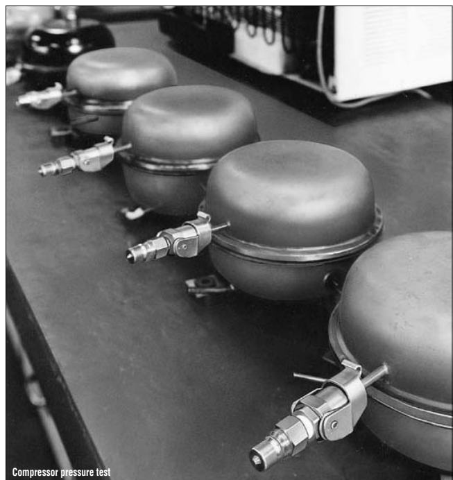
Compressor pressure test
