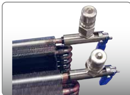
Helium Leak Test on Heat Exchangers
