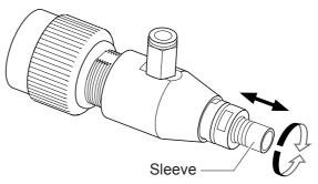
4 Use the attached two board spanners to fix the nut and moving sleeve Make sure the sleeve does not rotate.
