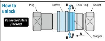
Slide the Lock Ring in the direction of the arrow A and rotate it in either direction simultaneously. When the Stopper is aligned with the deeper cutout on the Lock Ring, the Cupla will be unlocked.
