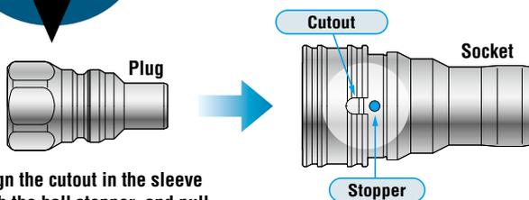
Align the cutout in the sleeve with the ball stopper, and pull the sleeve to connect the plug.
