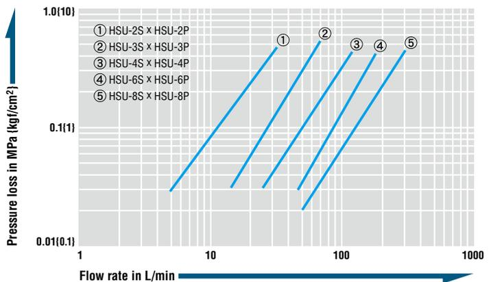
[Test conditions] • Fluid : Water • Temperature : 18°C
